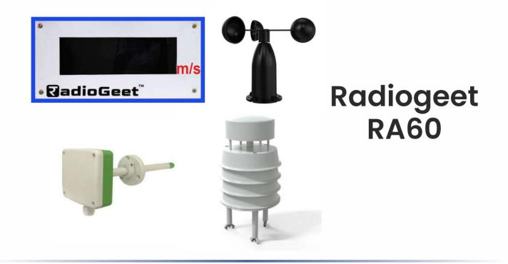
Model RA60 series are designed for highly accurate Wind Speed measurement for a wide range of industrial, pharmaceutical and building automation applications RA60 Model provides better than ±(0.2+0.03V) m/s accuracy. All these devices provide high performance in a compact design. 4-20 mA DC output signals can be fed as input to display. A rugged weather proof enclosure is available to monitor Wind Speed. A aluminum alloy material used for cup type anemometer.
